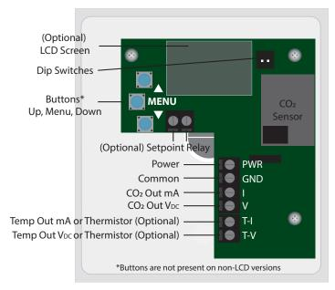
4. Set DIP switch positions to accomodate your application. DIP switch 2 only applies to units with transmitter temperature output selected.
